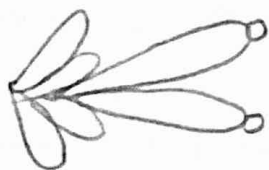
fig:- Switched Beamformer
